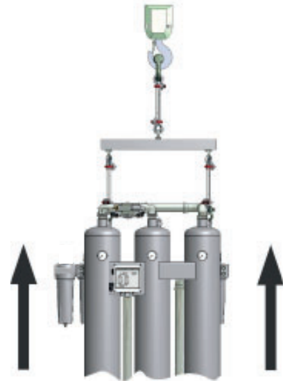
II: Installing by crane
